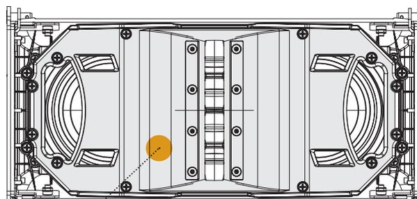
The frontal baffle's design increases the directivity of the line array doubling the radiation points on low/mid frequencies. The shape of the front baffle reduces the turbulence outside the waveguide decreasing the overall distortion.
